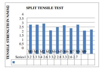
**Fig 4:** Graph shows 28 days of split tensile strength for normal concrete and concrete made with fly ash and GGBS as partial replacement of cement
