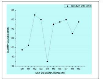
Fig 1: Graph shows slump values for normal concrete and concrete made with fly ash and GGBS as partial replacement of cement
