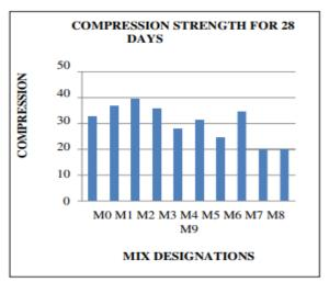
Fig 3: Graph shows 28 days compressive strength of normal concrete and concrete made with partial replacement of cement with fly ash and GGBS.
