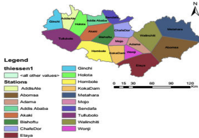
Fig 6: Thiessen polygons for the selected rainfall stations
