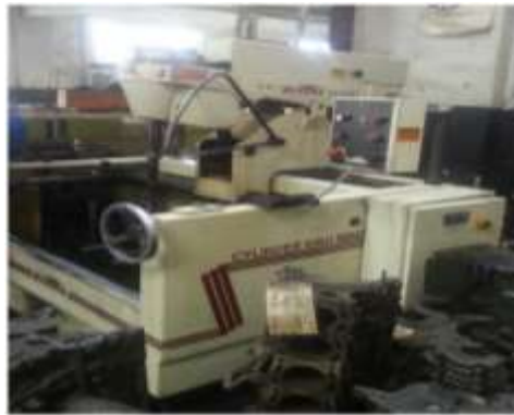
Figure 2. Sunnen CV-616 Cylinder King vertical honing machine
